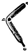
FIG. 51.—The liquefaction of ammonia in a thick bent tube. The compound of chloride of silver and ammonia is placed in the end a , and the end c is then sealed up.
